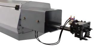
The first roller steady rest is mounted internally to the front of the bar feeder providing support to the bar as it enters the telescopic nose.
