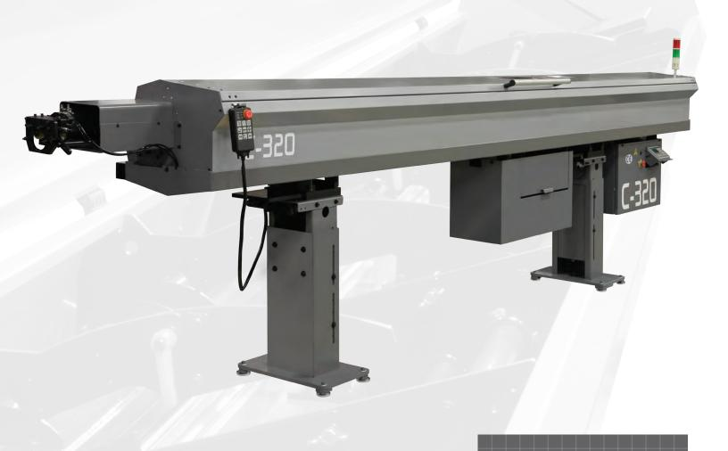
The C-320 is an Automatic Magazine style Bar Feeder designed for feeding round, square and hexagonal bar stock into Citizen CNC lathes.
