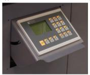
Alarms are well defined and displayed on the operator control panel. Panel swings out for ease of use.
